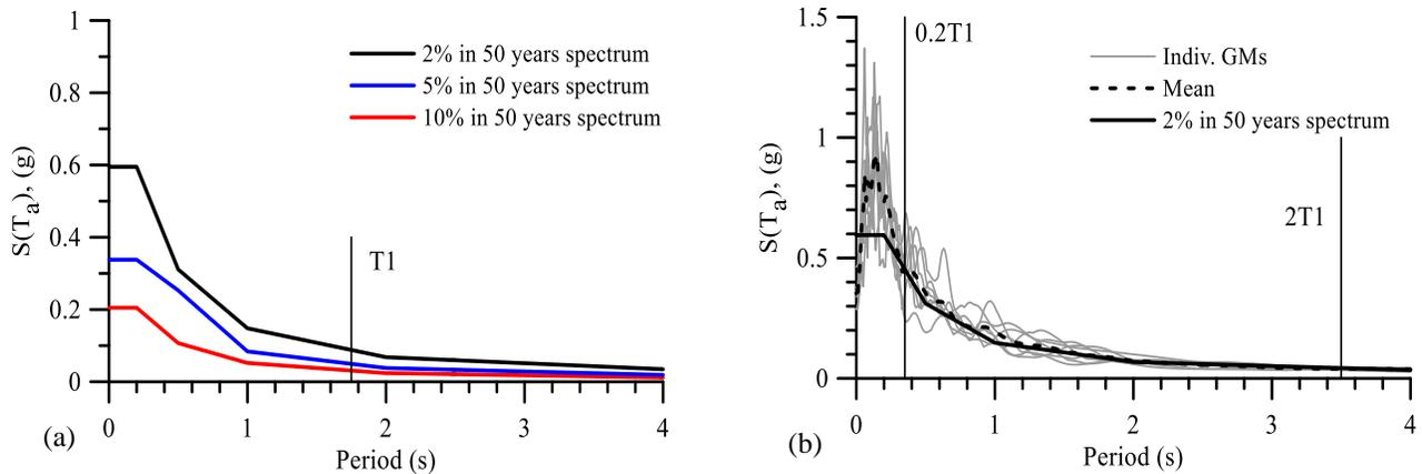
Figure 2. Response spectra: a) design spectrum and b) scaled response spectrum of selected records in the range  $0.2T_1 - 2T_1$
