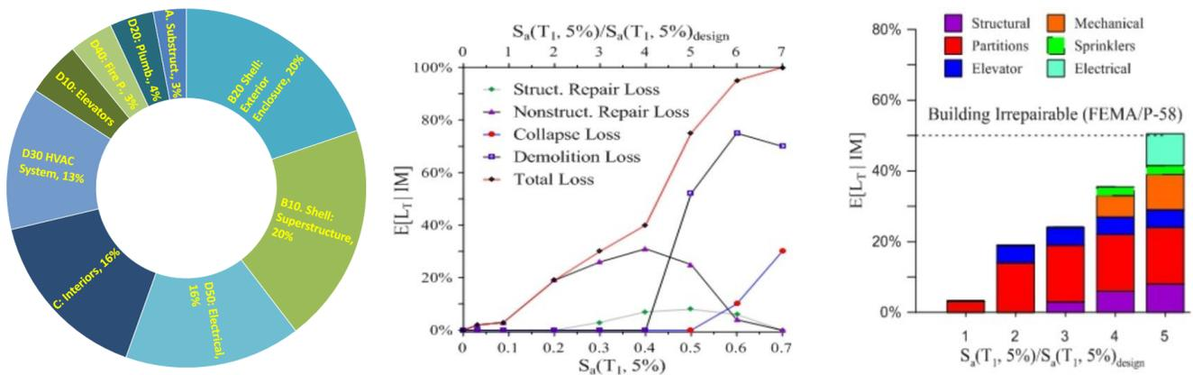
Figure 7. Earthquake loss estimation: a) distribution of building cost among its components, b) Loss-vulnerability curves for 8-storey MD-CBF building in Montreal, c) detailed distribution of % of building loss value at several  $IM$  levels
