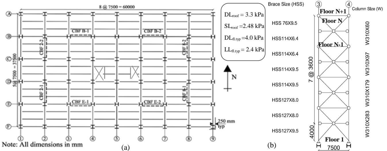
Figure 1. Building studied: a) floor plan and b) CBF1 elevation
