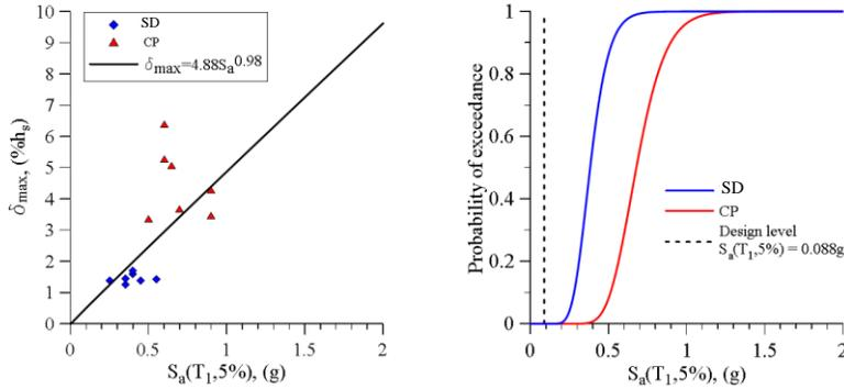
Figure 6. Seismic demand and the adjusted collapse fragility curve and severe damage fragility curve
