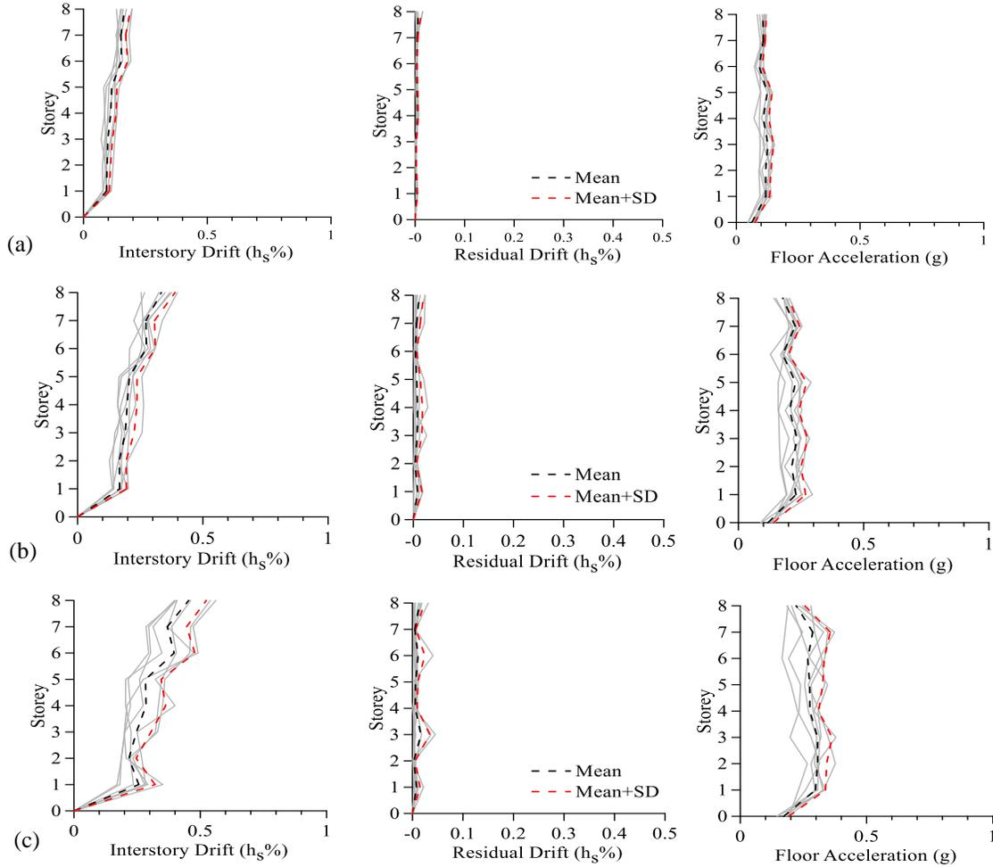
Figure 3. Nonlinear response of MD-CBF building with GMs scaled to: a) 10% probability of exceedance in 50 years; b) 5% probability of exceedance in 50 years; c) 2% probability of exceedance in 50 years (design spectrum)
