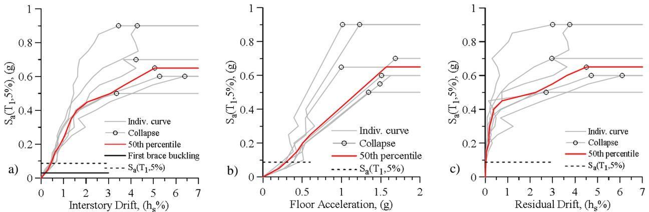
Figure 4. IDA curves of the 8-storey MD-CBF building computed in terms of: a) Storey drift; b) Floor acceleration, c) Residual storey drift.
