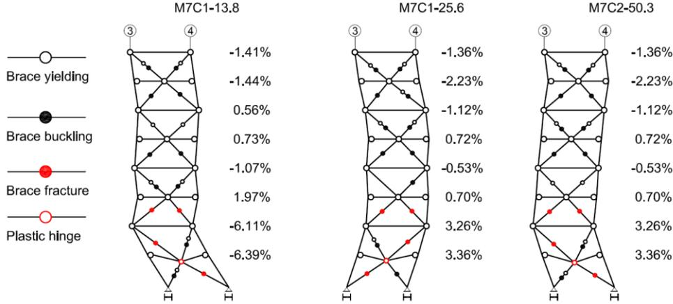
Figure 5. Failure mode of the studied 8-storey MD-CBF building
